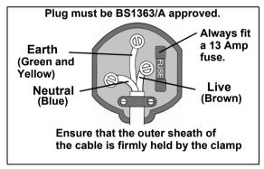
We strongly recommend that this machine is connected to the mains supply through a Residual Current Device (RCD)
